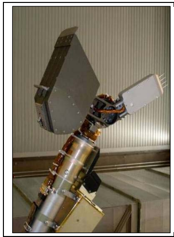
Figure 4-7: TECP (right) mounted on the robotic arm. The small white circle on the lower left is the humidity sensor. The four needles at right perform the other sensor measurements.
