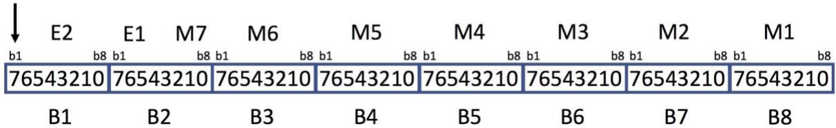
Fig. 5C-21. Double precision complex, most significant bytes (m-sign plus E2) first.
