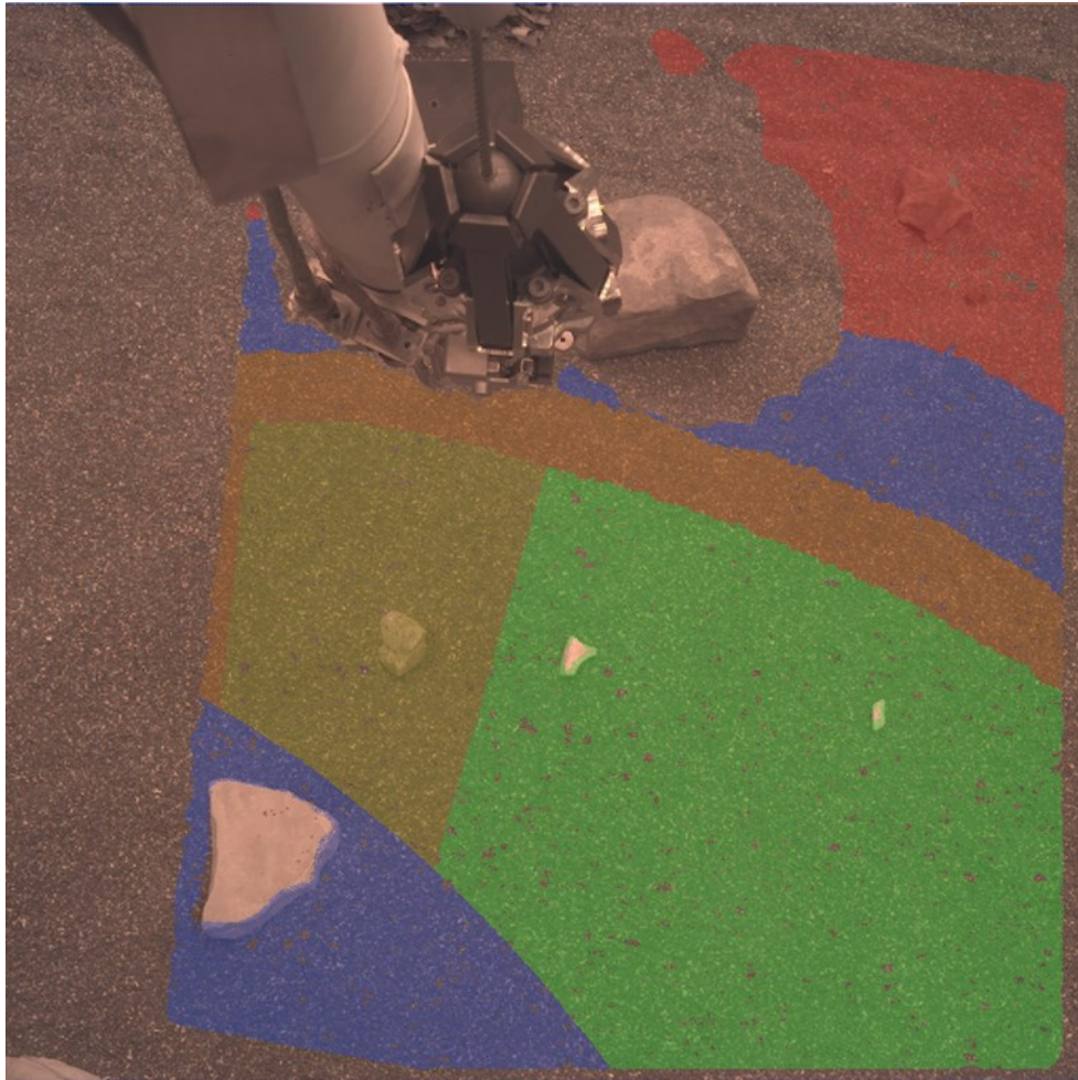
Figure 5-10: Workspace Reachability for HP3 (WSH) Data Overlaid onto Image EDR. Green indicates nominal zone for HP3 deployment (5), yellow is ICC partially occluded (6), orange is the kinematically reachable zone (4), blue is HP3 footprint boundary (2), and red is outside the HP3 boundary (1). Numbers refer to left column of Table 5-2.
