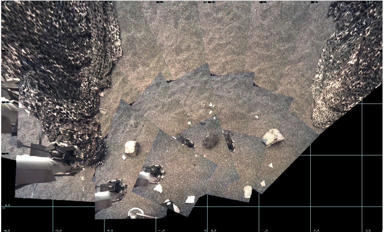
Figure 5-22: Vertical Projection Mosaic of Instrument Deployment Workspace. Arm is not masked off for purposes of illustration.
