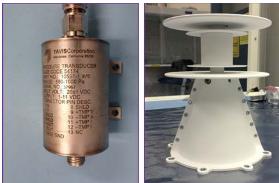
Figure 4.2.3.1-1: a) The Tavis Pressure Sensor and b) The Quad-Disc pressure sensor inlet.
