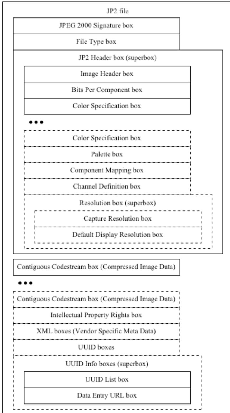
**Figure I.1 – Graphical representation of a JP2 file. Dashed lines indicate optional boxes. (Modified from ISO/IEC 15444-1:2004, “Information technology – JPEG 2000 image coding system: Core coding system”, figure T.800\_FL1)**
